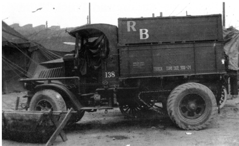
Photo 2 - RBBB No. 138 in a later photo now sports a tank body. Note the reinforcing on the tank and the boarded storage area above the tank. Also note the Power-Take-Off (PTO) driven pump mounted on the running board with a discharge pipe routed under the door and over the fender with a hose folded back over the fender. [Wm. Koford Collection]
