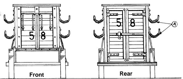
All pole racks are wrapped with rope (See Detail "A"
