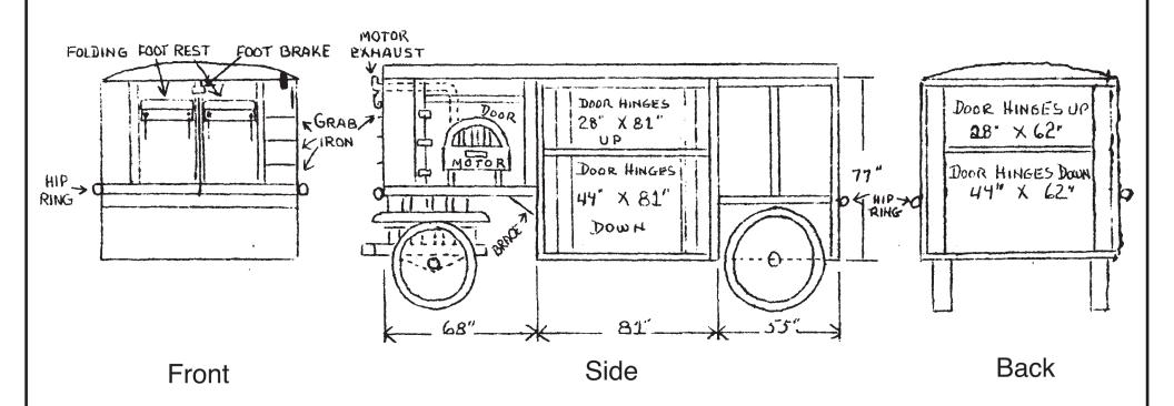
Specifications: Length 17' Width 88" Height 7' Door to Motor Size 38 1/2" X 56"
