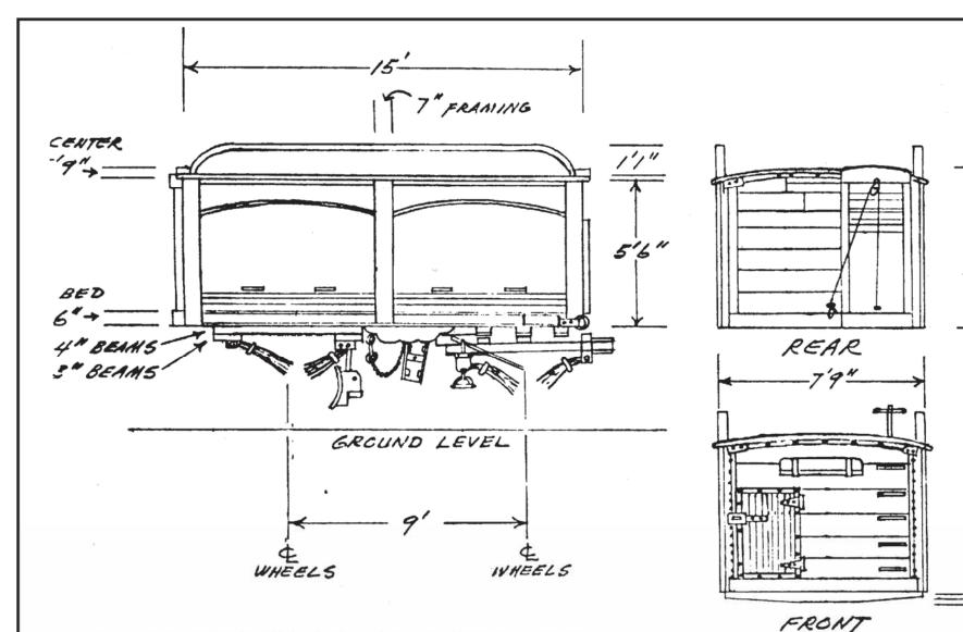
This wagon will take 2'9" wheels in front and 3'3" wheels on the rear. (Schmidt small wheels) (DRILL OUT HUBS & REPLACE WITH "GLOBE" HUBS.
