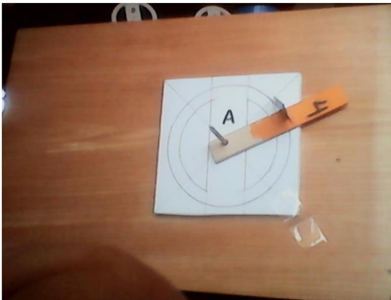
Start with a piece of 3/16 foam board. Using a piece of wood with a notch cut into it, the inside and outside dimension of the rim, cut on both side of the foam board, side A and side B. NOTE on side A do not cut in the middle of the two straight lines
