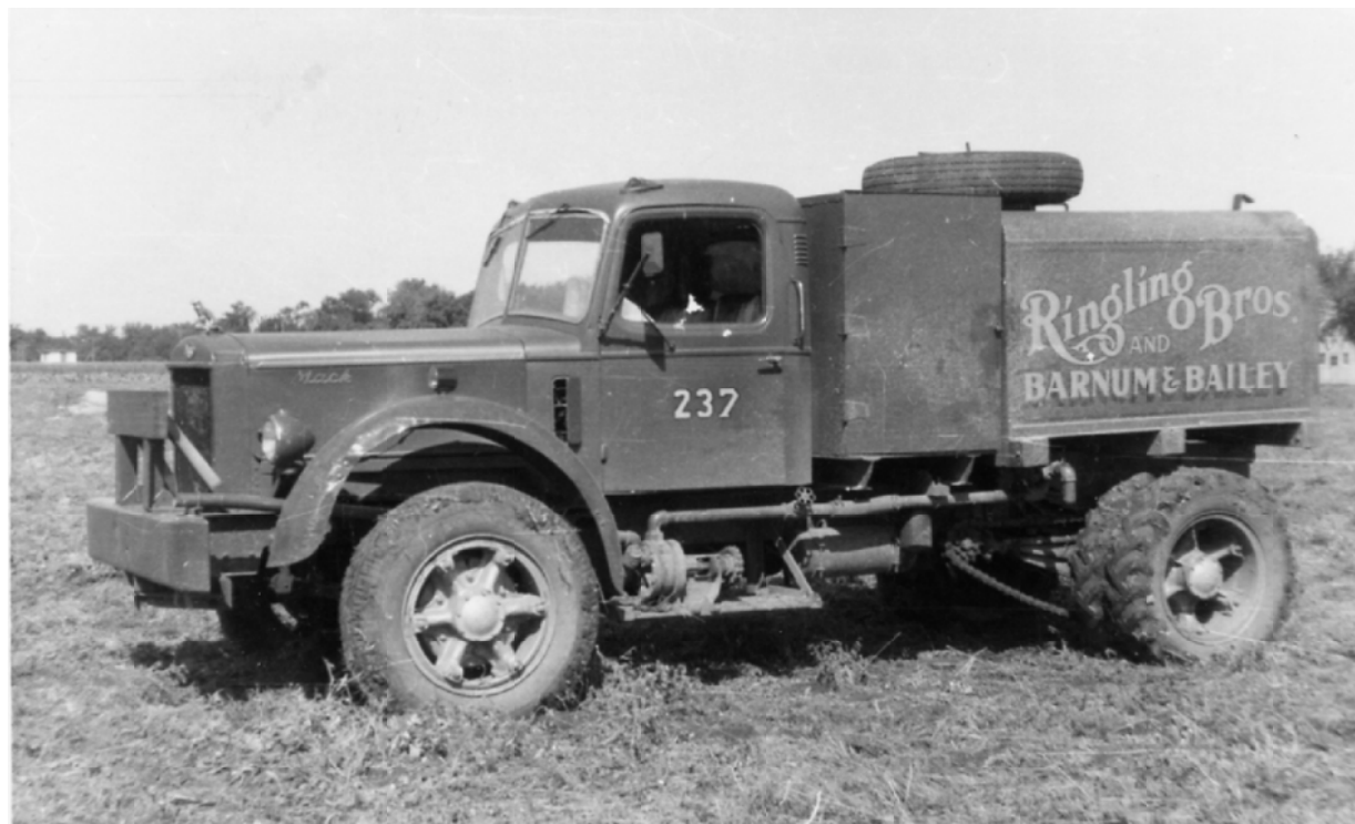
Photo #1- Left side of #237. Note water pump mounted under driver’s side of cab on running board. Short high water tank with storage box in between cab and tank. Spare tire mounted on top. [Photo from M. Dreiling Collection]
