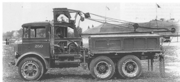
#250 Mack in 1935. Note detail of the crane super structure, air tanks, jackscrew stabilizer and the doors on stock supply box.
