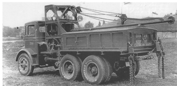
#250 in 1935 detail of boom holder, piles, cables, rear doors, two rings on end of frame and spreader chains.
